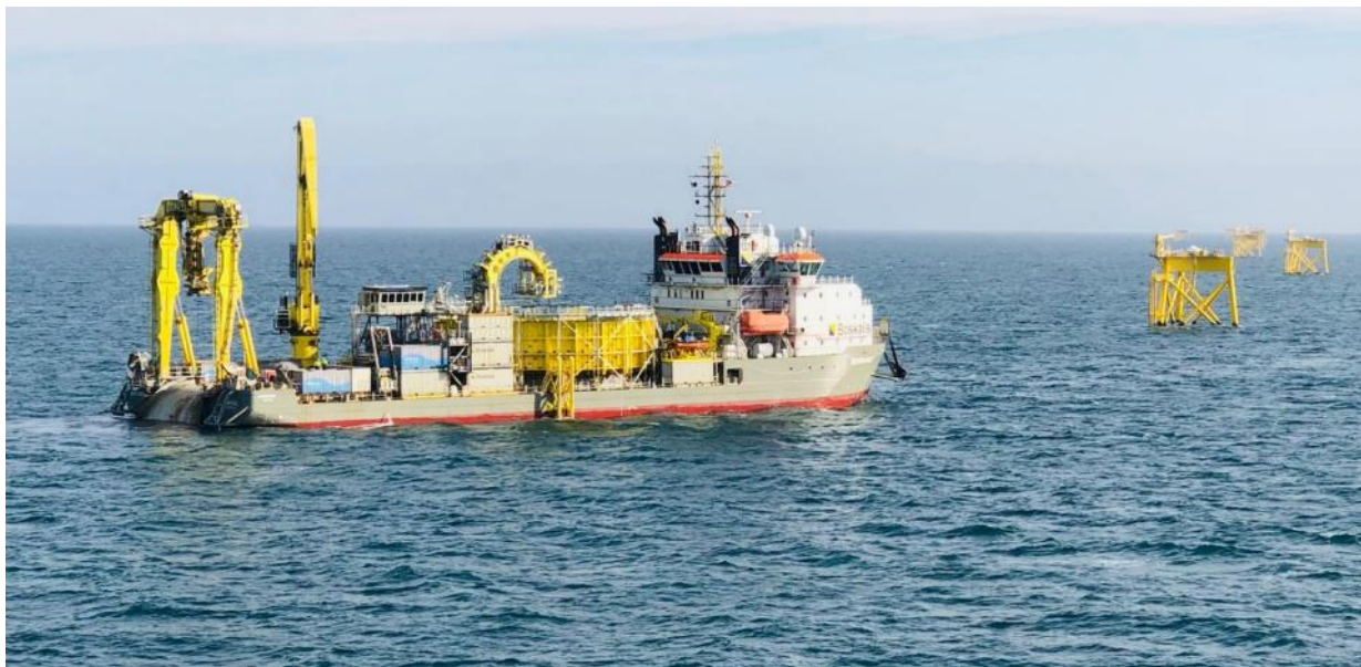
Plate 6.15 Cable Laying Vessel Operating at the East Anglia ONE Windfarm Site
