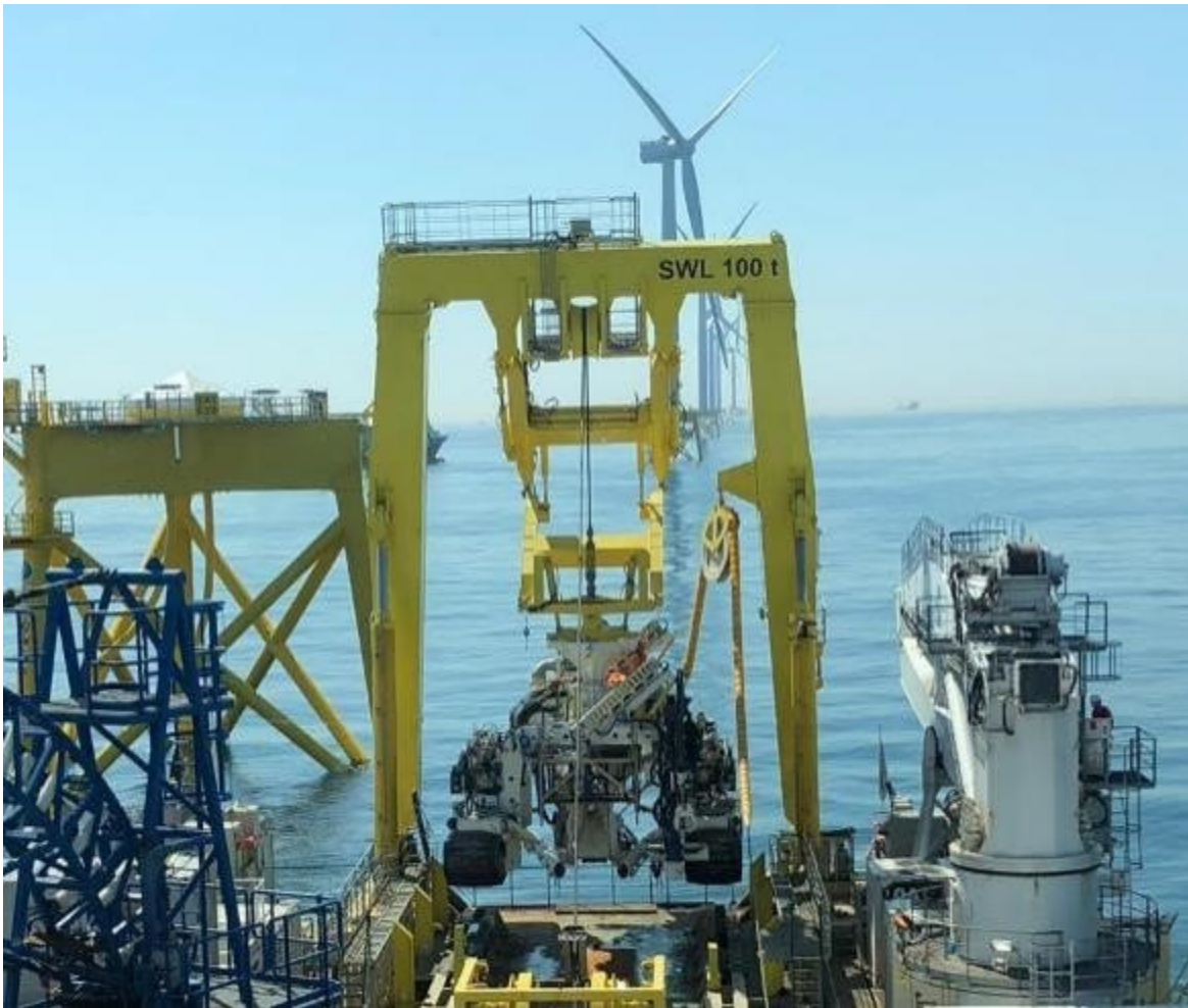
Plate 6.14 Photo of an indicative plough trencher (the likely installation method for platform link and inter-array cables)
